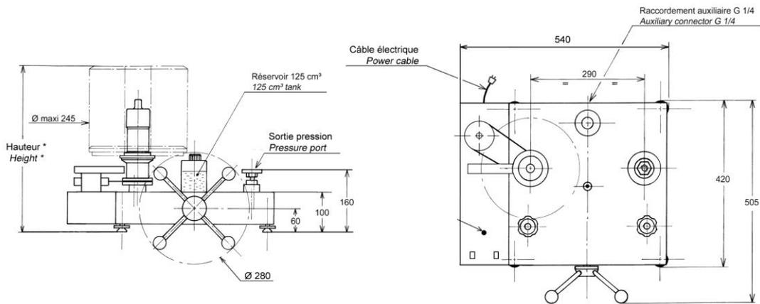
Height with standard set of weight : (bar, KPa) : 450 mm
