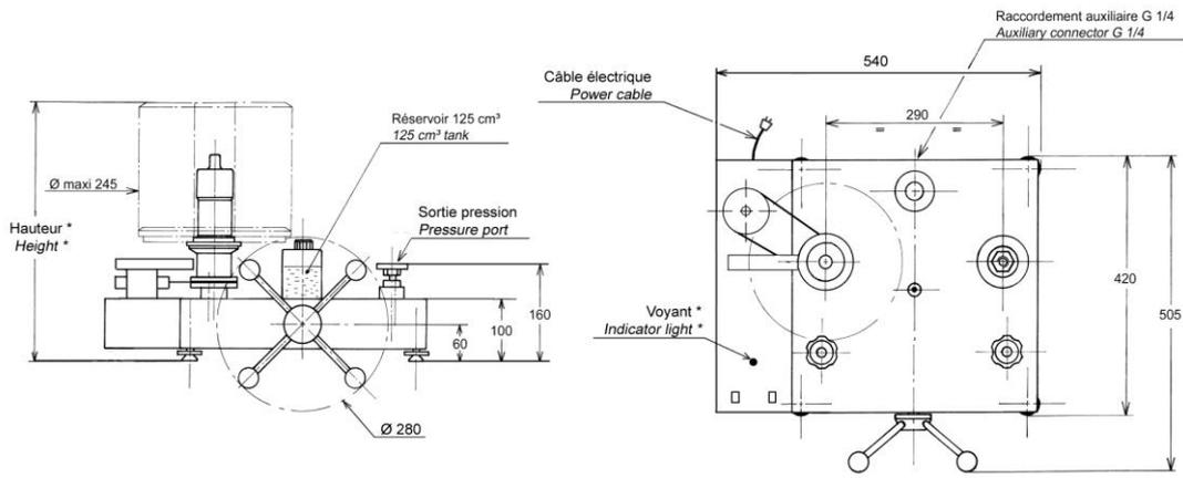
Height with standard set of weight : (bar, KPa) : 340 mm (PSI) : 350 mm
